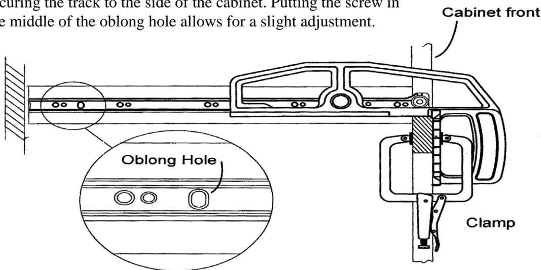
When building frameless cabinets or when the cabinet side is flush with the inside edge of the stile the cabinet track can be screwed to the inside of the cabinet as shown in the bottom left drawing.
