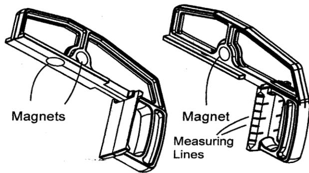
This tool's design employs magnets to hold the cabinet track in place. The new magnetic design improves the ease of use of this tool. There is a magnet on each side of the Drawer Slide Mounting Tool so one tool is used for mounting the track to the cabinet on either side of the drawer.
