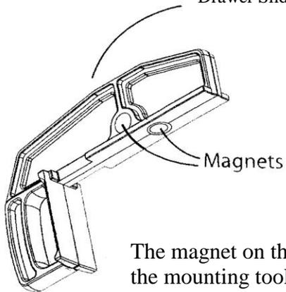
The magnet on the bottom of the mounting tool is used to locate bottom mount drawer slide as shown on the right.
