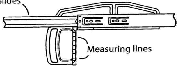
Full extension drawer slides are designed to support a lot of weight and extend all of the way out of the cabinet. The Drawer Slide Mounting Tool is ideal for accurately positioning full extension drawer slides.
