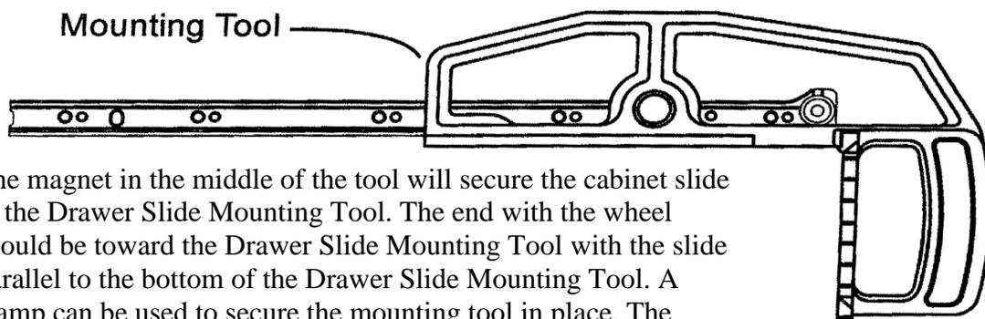
The magnet in the middle of the tool will secure the cabinet slide to the Drawer Slide Mounting Tool. The end with the wheel should be toward the Drawer Slide Mounting Tool with the slide parallel to the bottom of the Drawer Slide Mounting Tool. A clamp can be used to secure the mounting tool in place. The cabinet track typically has an oblong hole. Use this hole for securing the track to the side of the cabinet. Putting the screw in the middle of the oblong hole allows for a slight adjustment.
