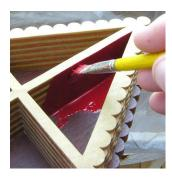
Flock It! Suede-Tex undercoat adhesive can be **brushed**, **sprayed or rolled** onto the area to be coated.
