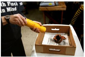
Hold the outer tube (printed one) with one hand; twist the inner tube (see photo above) while pumping to spray the object you wish to coat. Keep the Mini Flocker 8" to 10" from surface and as close to 90 degree to the object as possible.
