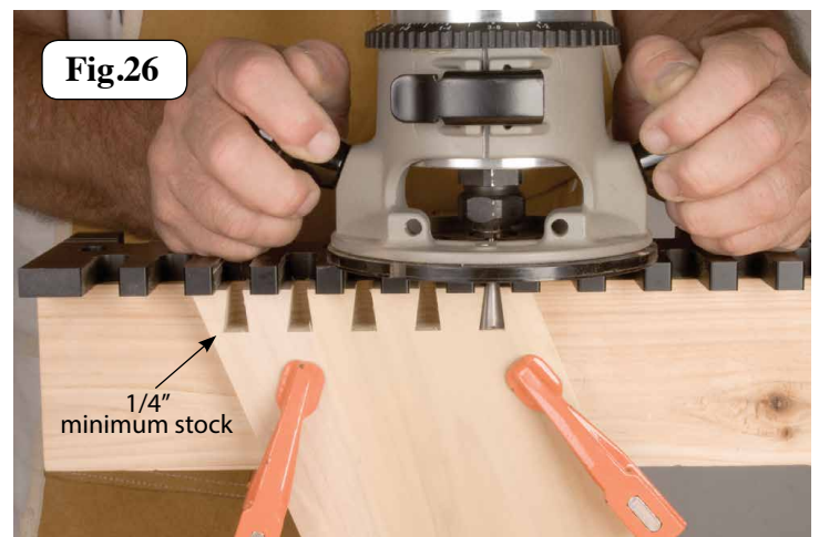
The example above shows the correct spacer attached to the original mounting block for cutting 1/2" stock using the small router bit set.
